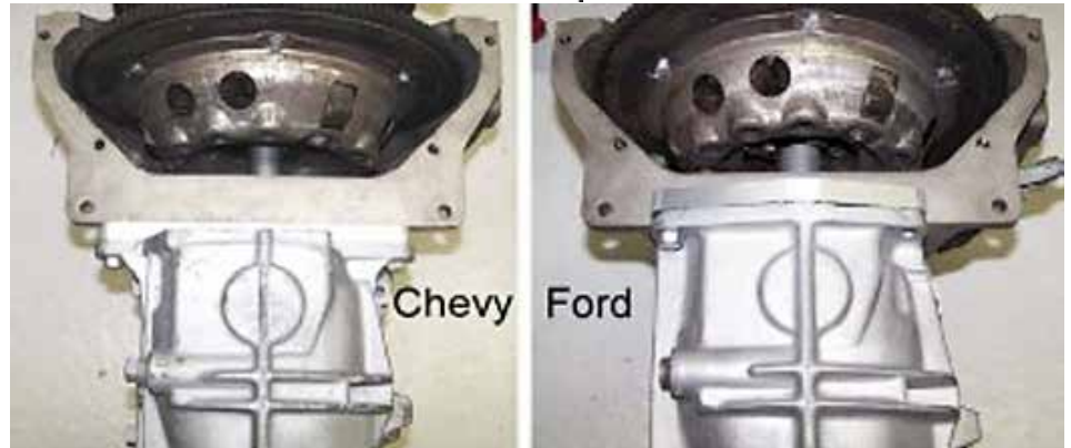
Adapter installed on Flathead Bellhousing.
